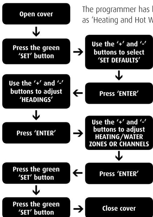
The programmer has been preset to display the channel heading as 'Heating and Hot Water', should you require either the 'Zone' or 'Channel' options then please follow the flowchart opposite.
