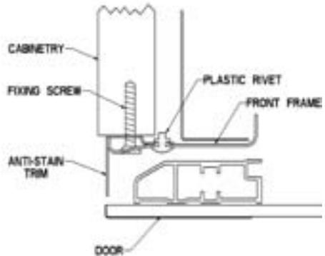
Note : When supplied the anti-stain trim may be loose and is only supported by plastic rivets. The anti-stain trim will be secured when the fixing screws are fully home into the cabinet. The plastic rivets should not be removed.
