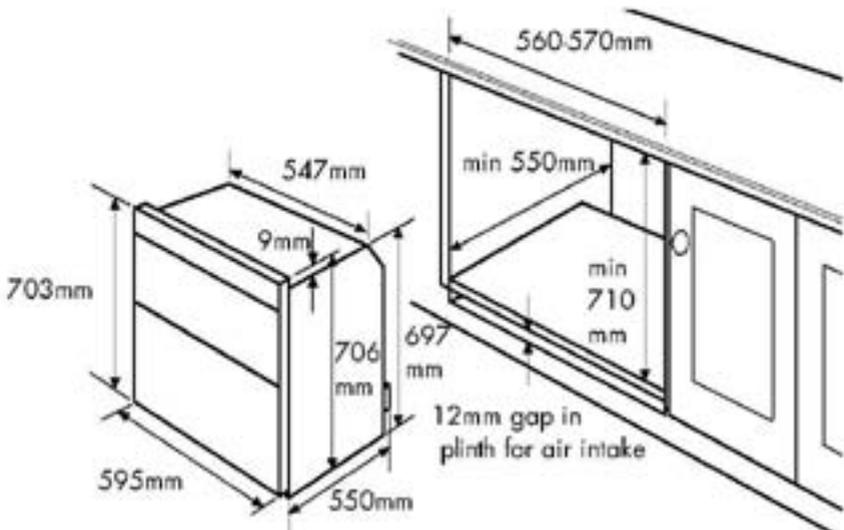
1. When installed in a typical 600mm deep built in housing unit, the false back should be removed from the housing unit to provide the necessary depth for installation.
